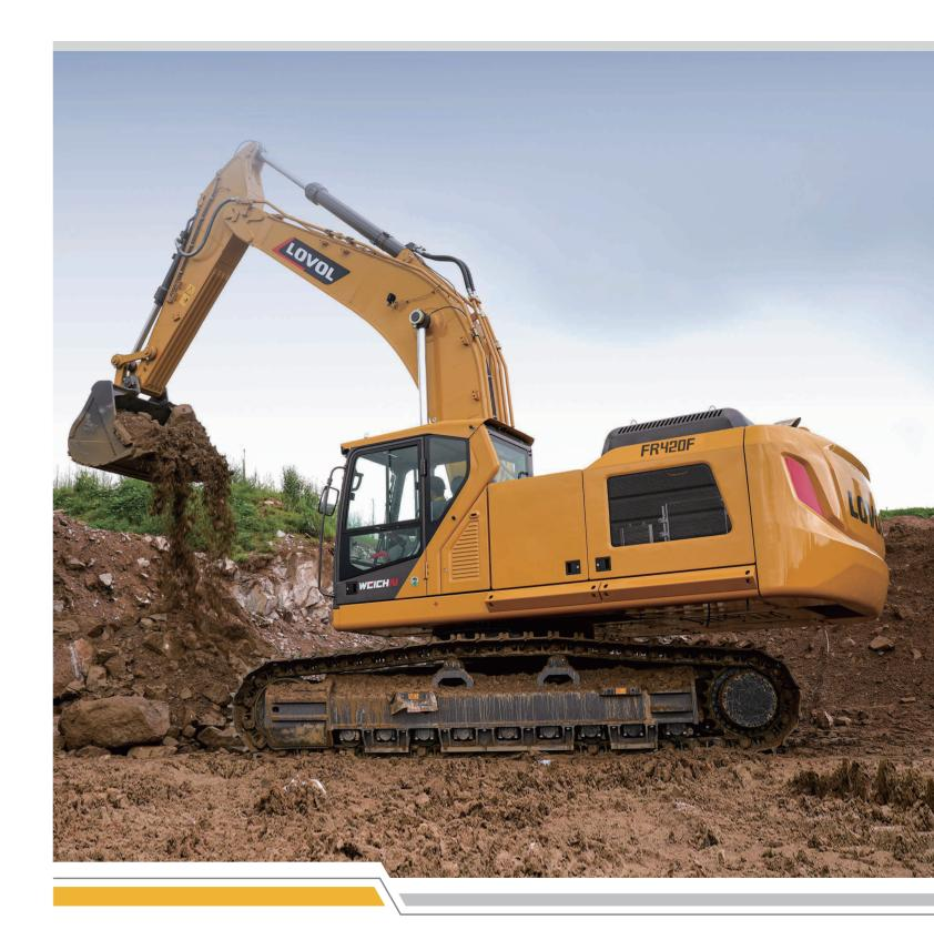
Rated Power Operating Weight Bucket Capacity 247kW/2000rpm 41500kg 2.2m<sup>3</sup>
